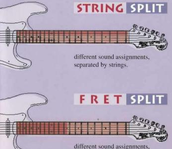
different sound assignments, separated by fret, plus Hold Pedal function for an additional sound.
