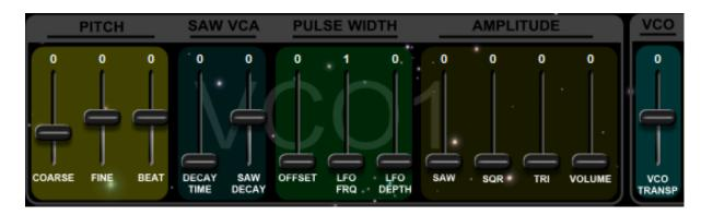
The FI contains four identical Voltage-Controlled Oscillators (VCOs) and these provide the basic sound source for the synthesizer. Each oscillator has three waveforms (saw, square and triangle) which can be used simultaneously. The sliders in this block adjust the tuning, volume and character of the oscillator. The oscillator blocks are located on the left-hand side of the Editor screen and, moving from left to right, their sliders are as follows:
