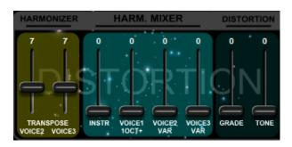
The Distortion Block applies distortion to the original instrument signal and to the three transposed voices generated by the Harmonizer. VOICE1 is fixed at 1 octave above the input signal, whereas the transpositions of VOICE2 and VOICE3 are variable.
