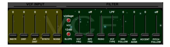
The Voltage-Controlled Filter (VCF) is one of the most important sound-shaping tools in a synthesizer. Basically it removes certain frequencies from a sound, thus altering its harmonic content. Depending on the type of filter used, the frequencies *above*, *below* or *at* a specified "cutoff" frequency are removed. This cutoff frequency can be modulated dynamically from different sources (e.g. an envelope), thus creating sounds which evolve over time.
