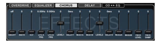
This effect is very flexible; in addition to Chorus, it can be configured as a Flanger, Slapback Echo or simple Reverb merely by setting the parameters differently.
