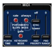
The parameters in this block are relevant only if the FI4 is being played using its MIDI IN port or if it is being synchronized to a MIDI clock signal via the MIDI IN port.
